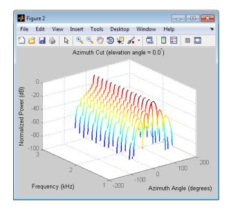
Apply a subband phase shift beamformer to the array. The direction of interest is 30 degrees azimuth and 0 degrees elevation.
