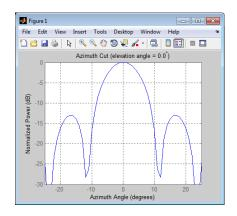
Assume that you have two signal sources with DOAs separated by ten degrees. Because both DOAs fall inside the main lobe of the array response, the beamscan DOA estimator can not resolve them as separate sources.
