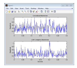
The adaptive beamformer significantly improves the SNR of the rectangular pulse at 0.2 s.
