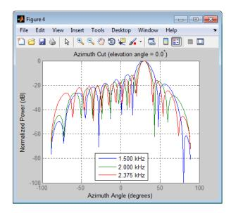
This plot shows that the main beam direction remains constant, but the beam width decreases with frequency.
