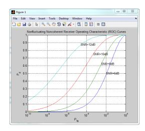
The graph shows that—as the SNR increases—the supports of the probability distributions under the null and alternative hypotheses become more disjoint. Therefore, for a given false-alarm probability, the probability of detection increases.
