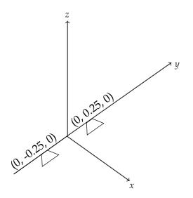
The elements are located 0.25 meters from the phase center of the array and the distance between the two elements is 0.5 meters.
