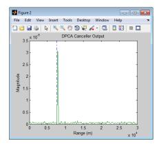
The DPCA pulse canceller has significantly rejected the clutter. As a result, the target is visible at the expected range gate.
