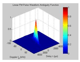
The surface has a narrow ridge that is slightly tilted. The tilt indicates better resolution in the zero delay cut. For a more detailed analysis of waveforms using the ambiguity function, see Waveform Analysis Using the Ambiguity Function.
