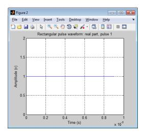
plot is a method of phased.RectangularWaveform. This plot method produces an annotated graph of your pulse waveform.
