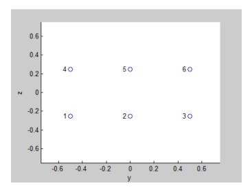
Create an array consisting of three 2-element linear subarrays parallel to the *z*-axis. Use the numbers in the plot to help form the matrix for the SubarraySelection property. Also, find the phase centers of the three subarrays.
