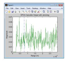
Apply the adaptive DPCA pulse canceller. Use 100 training cells and 4 guard cells, two on each side of the target range gate.
