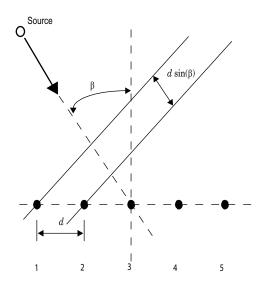
Because of the angle of arrival, the array elements are not simultaneously illuminated by the plane wave. The additional distance the incident wave travels between array elements is  $d \sin(\beta)$  where *d* is the distance between array elements. Therefore, the constant time delay between array elements is:
