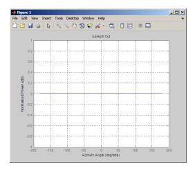
Setting the BackBaffled property to true limits the response to azimuth angles in the interval [-90,90].
