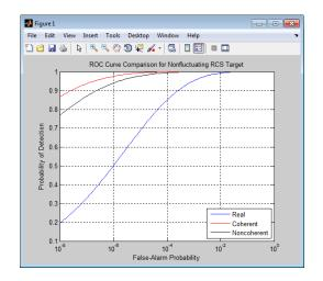
The ROC curves clearly demonstrate the superior probability of detection performance for coherent and noncoherent detectors over the real-valued case.
