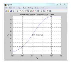
The ROC curve enables you to easily read off the probability of detection for a given false-alarm rate.
