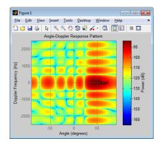
As expected, the angle-Doppler response shows the greatest response at zero Doppler and 45 degrees azimuth.
