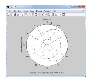
Calculate the microphone's response at 30 degrees and 60 degrees azimuth with corresponding elevation angles of 0 degrees.
