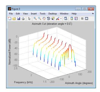
The plot shows the beamformed pattern at the center frequency of each subband.
