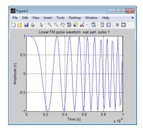
Use the step method to obtain your pulse waveform signal. Plot the real and imaginary parts of one pulse repetition interval.
