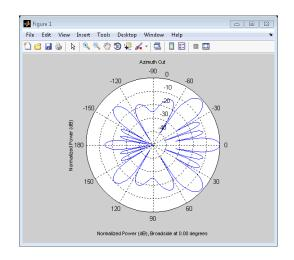
By default, plotResponse shows the array's normalized power response in decibels (dB) at zero degrees elevation for azimuth angles from [-180,180]. You can view azimuth cuts of the array response from various elevation angles and elevation cuts from various azimuth angles by specifying name-value pairs in plotResponse.
