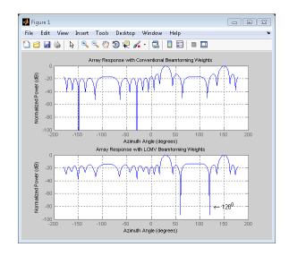
The LCMV beamforming weights place a null in the array response at the arrival angle of the interference signal.
