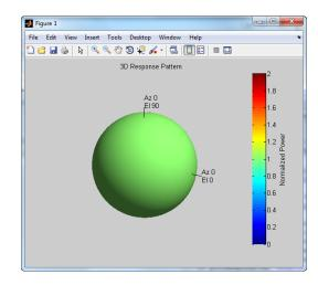
${\tt plotResponse}$  is a method of phased.IsotropicAntennaElement. By default,  ${\tt plotResponse}$  plots the response of the antenna element in decibels (dB) at zero degrees elevation.
