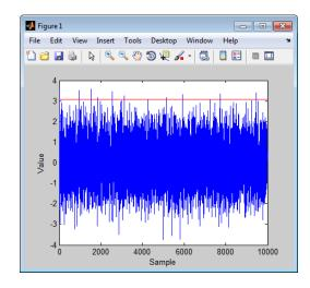
The red horizontal line in the plot indicates the threshold. You can see that few sample values exceed the threshold. This result is expected because of the small false-alarm probability.
