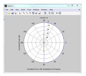
Use step to obtain the microphone's magnitude response at the specified azimuth angles and frequencies. The elevation angles are 0 degrees. Note the response is one at all azimuth angles and frequencies as expected.
