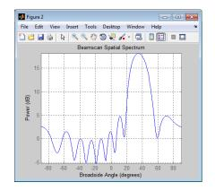
The beamscan estimator does not resolve the two sources based on their DOAs.
